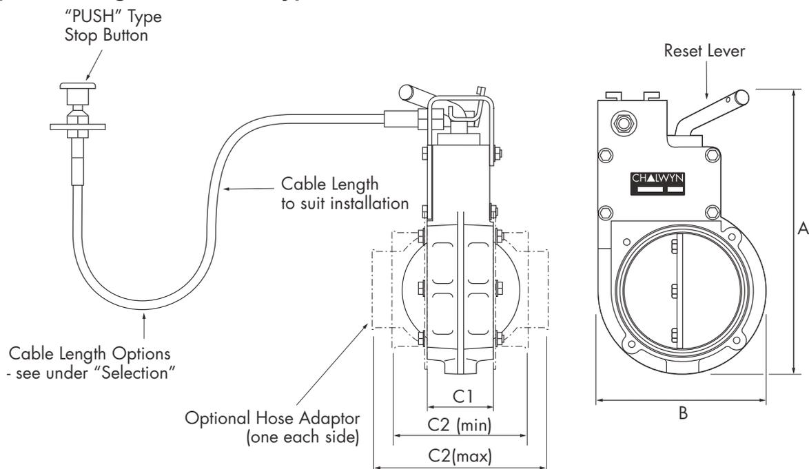
**Typical Arrangement: Valve Types MVX-303, MVX-503 and MVX-803**
